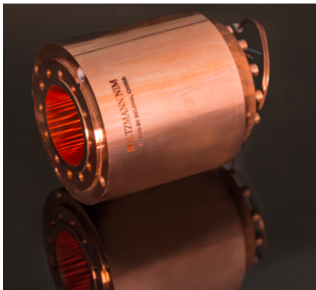
Figure 2 - NIM cylindrical acoustic gas thermometer used to measure the Boltzmann constant
